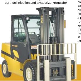
to convert the fuel from a liquid to a gas for vapor injection. The Engine Control Unit electronically regulates the fuel, air, and spark advance to provide the necessary torque. The engine control unit's inputs include manifold air pressure, manifold air temperature, engine coolant temperature, accelerator pedal position, throttle position, engine speed, cam signal, and oxygen sensor signal.
