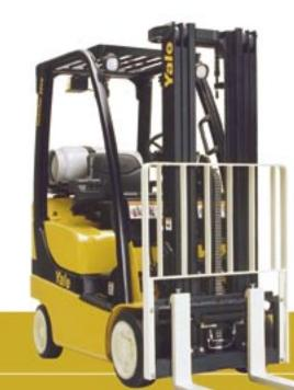
There are two transmission selections available that will handle a wide variety of material handling applications. Both transmissions feature electronic inching (requires no overlap adjustment), electric shift control, neutral start switch, and anti-restart protection. A single pedal controls both inching and braking. Optional dual inch/brake pedals are available for operators who prefer this design. A 10 micron filter protects the transmission from abrasive contaminants.
